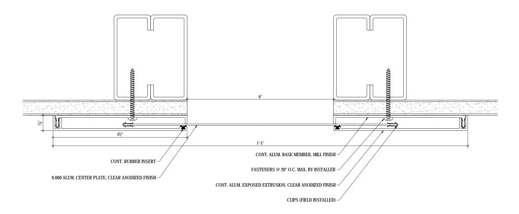
NOTE: 1 HOUR CONSTRUCTION INDICATED 2 LAYERS OF GYPSUM BOARD FOR 2 HOUR CONSTRUCTION
